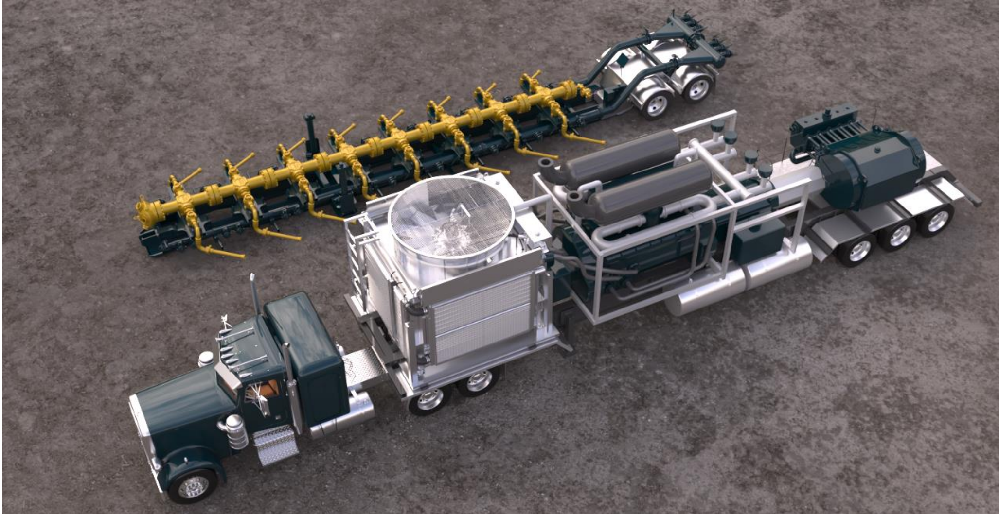
ICBM Manifold Trailer, Jumbotron Radiator, Power End
